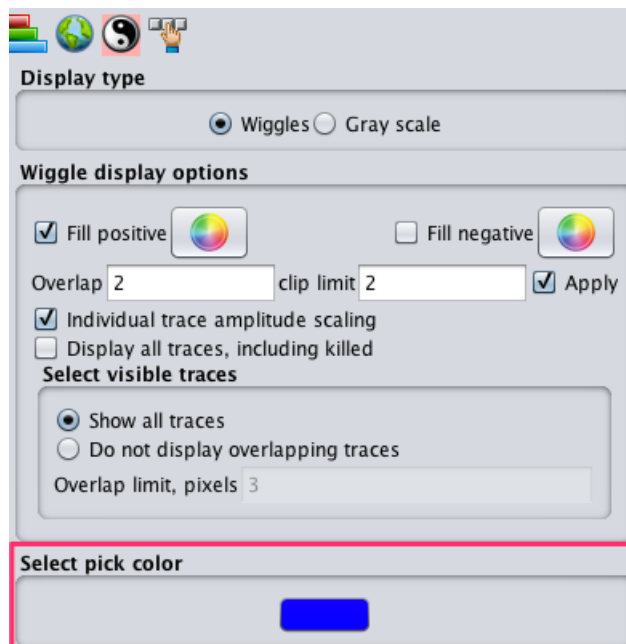
Figure 6---50 Wiggle display options, highlighting the Select pick color option.
